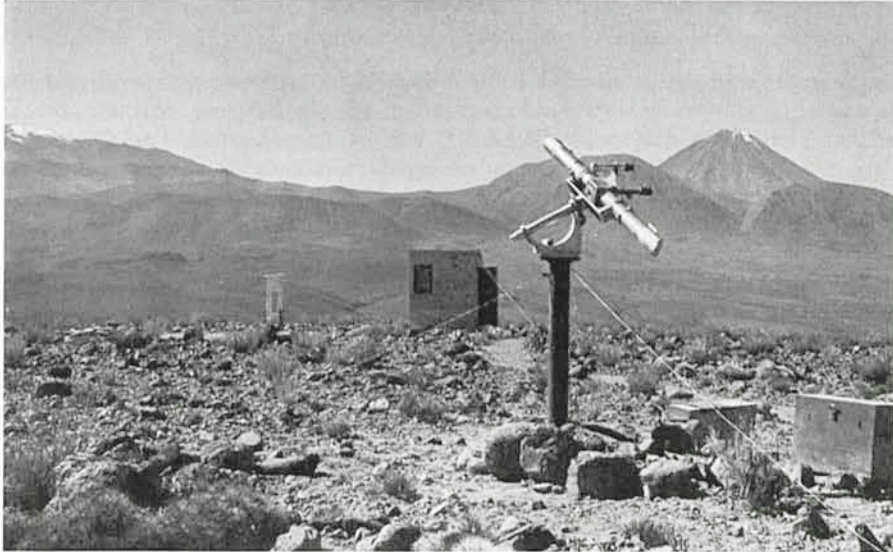
Fig. 3: Double-beam telescope on Cerro Chaupiloma. In the background the volcano Licancabur.
