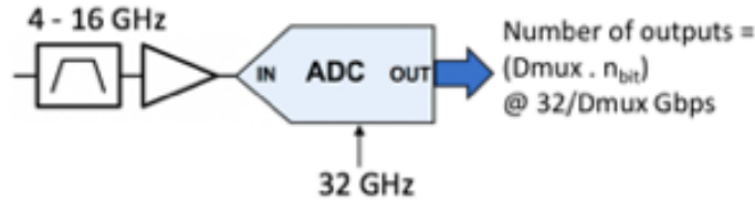
Figure 41: Direct sampling for an IF range between 4 and 16 GHz, assuming that the ADC chip includes a demultiplexed output. The 4-16 GHz range is taken as an example and brings new science capabilities.
