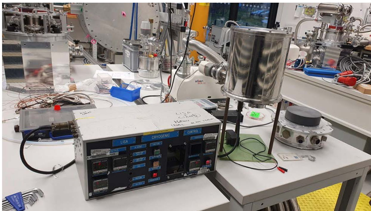
Picture: Broadband CCD bath cryostat under test at ESO.© ESO
