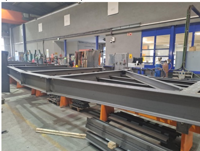
Figure 7: Sub-Nasmyth platform in production in Germany before shipment to Chile
