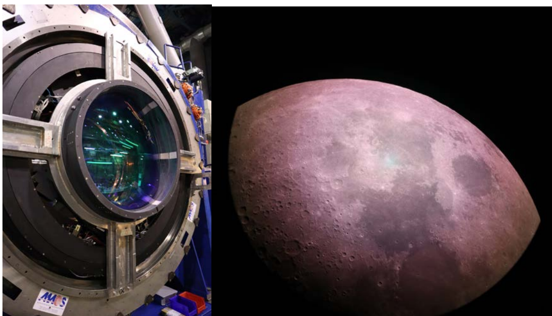
Figure c) the corrector mounted on UT1 and the first light image, projecting onto a screen. The Moon appears red because the anti-reflection coating is optimised for the red and IR, not the blue.
