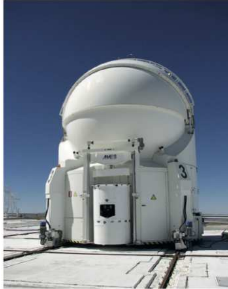
Figure 4. An auxiliary Telescope with the lifted ROS module ready to be moved to a different baseline position.
