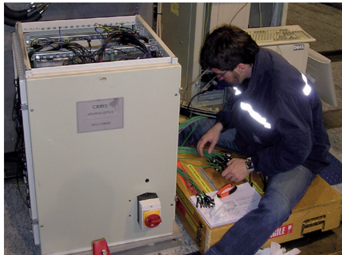
Figure 1b: A team member, trying to sort out and re-connect the fibre bundle connecting the wave-front sensor lenslet array with the 60 avalanche photo diodes (APDs) contained in a special cabinet. The APDs are solid-state photon-counting detectors. As curvature wavefront sensing systems basically need only one fast photometric channel per sub-pupil, APDs were given preference over CCD-detectors, due to their extremely low noise level (typically 0.4 counts per loop cycle). APDs, however, are very sensitive and fragile devices, and the prevention of accidental (and catastrophic) overexposures is a key issue.
